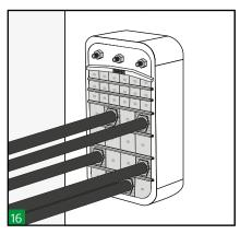
Make a visual inspection of the transit. Hawke's unique colour coding system enables the installation to be visually inspected after completion and ensures correct matching of the block halves. Check that marks in all the cables are visible to be guarantee blocks and cable copper tapes are aligned.
