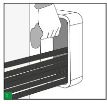
Make sure the frame is clean, then pull cables or pipes through, placing the largest at the bottom. (Note: Use open ended frame to fit around existing cables/pipes)
