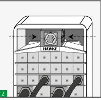
Compression tool must be introduced centered in the frame both in width and depth since otherwise the compression of the system would not be balanced so that to be able to introduce the lateral pieces of the endpacker t it would be necessary to over tighten the tool and it could be damaged.
