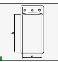
Before using the compression tool, it is important to check that the complete sealing area of this frame size (see table) is filled with blocks. Thus over tightening of the tool can be avoided.
