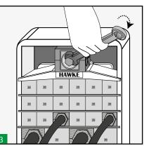
Once centered, we begin to tighten the compression tool which will be pressing on the compression plate.
