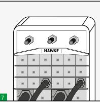
Tighten the nuts on the endpacker alternately following the above sequence to compress and complete the seal. Use a ratchet spanner for an easier installation. Approximately 10-12 mm of thread should protrude on each bolt to ensure the sealing.  $\rightarrow$  Recommendations of good use.
