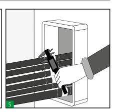
Take measures of cables diameters and select the appropriate Hawke tolerant blocks.
