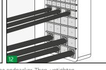
Insert the outer blocks of the endpacker. Then, untighten the compression tool and remove it.
