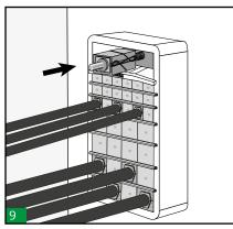
Pack the last row between the last stayplate and the compression plate. Insert the compression tool on the top, in the centre of the compression plate.
