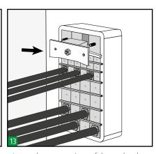
Insert the centre piece of the endpacker along with the front plate.
