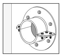
Check that Hawke Sleeve has been used in the istallation, that it has been properly installed (welded/bolted) and that is has not mechanical or corrosion damage.
