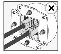
Check the correct orientation of the blocks.
