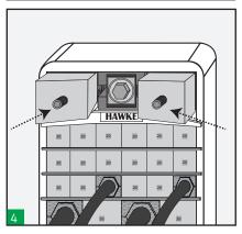
Before reaching the limit of tightening we must check if we have enough space to introduce the endpacker lateral pieces to avoid over tightening the tool that could block it.
