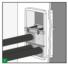
Clamp Tool can be used to fix blocks in their place when the transit installation is not completely finished.
